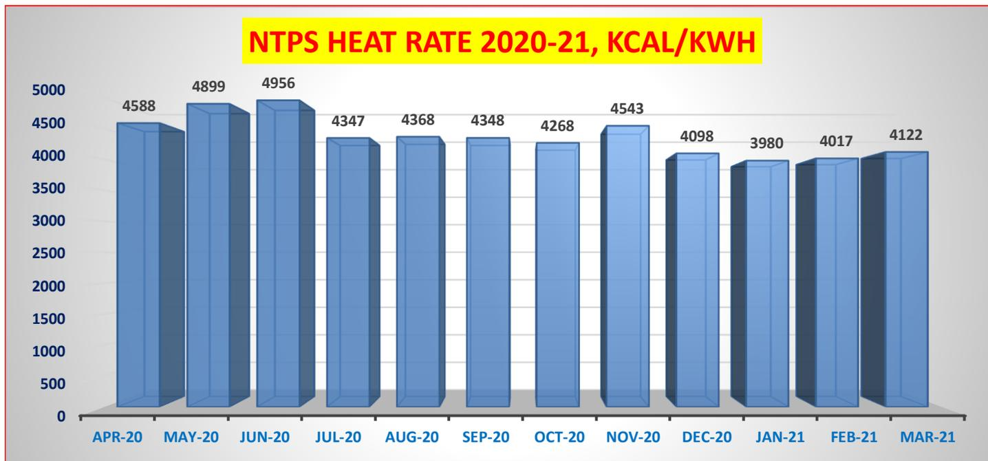
Observation : Heat rate for NTPS for the year 2020-21 is depicted in above chart. Heat rate is observed to be varying from 3980kcal/kWh to 4965 Kcal/kWh. Heat rate is found to be highest in the month of Jun 20 and lowest in the month of Jan 21 .
