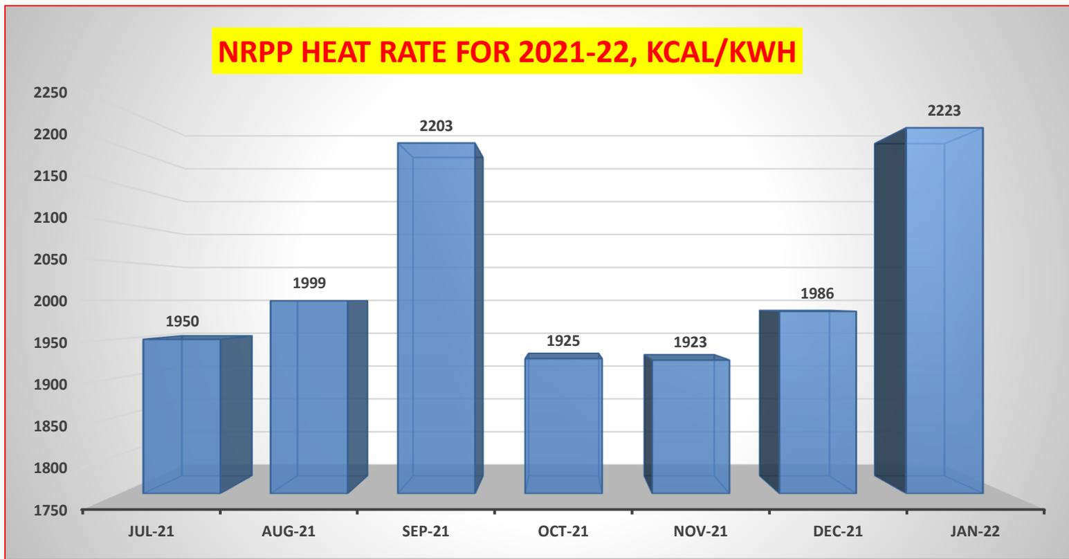
**Observation :** Heat rate of NRPP for the year 2021-22 is depicted in above diagram. Heat rate is observed maximum in the month of January 2022 i.e., 2223 kCal/kWh and minimum in the month of November 21 i.e., 1923 kCal/kWh . the Average heat rate for the year 2021-22(Upto January 20220 is found to be 2030 kCal/kWh.
