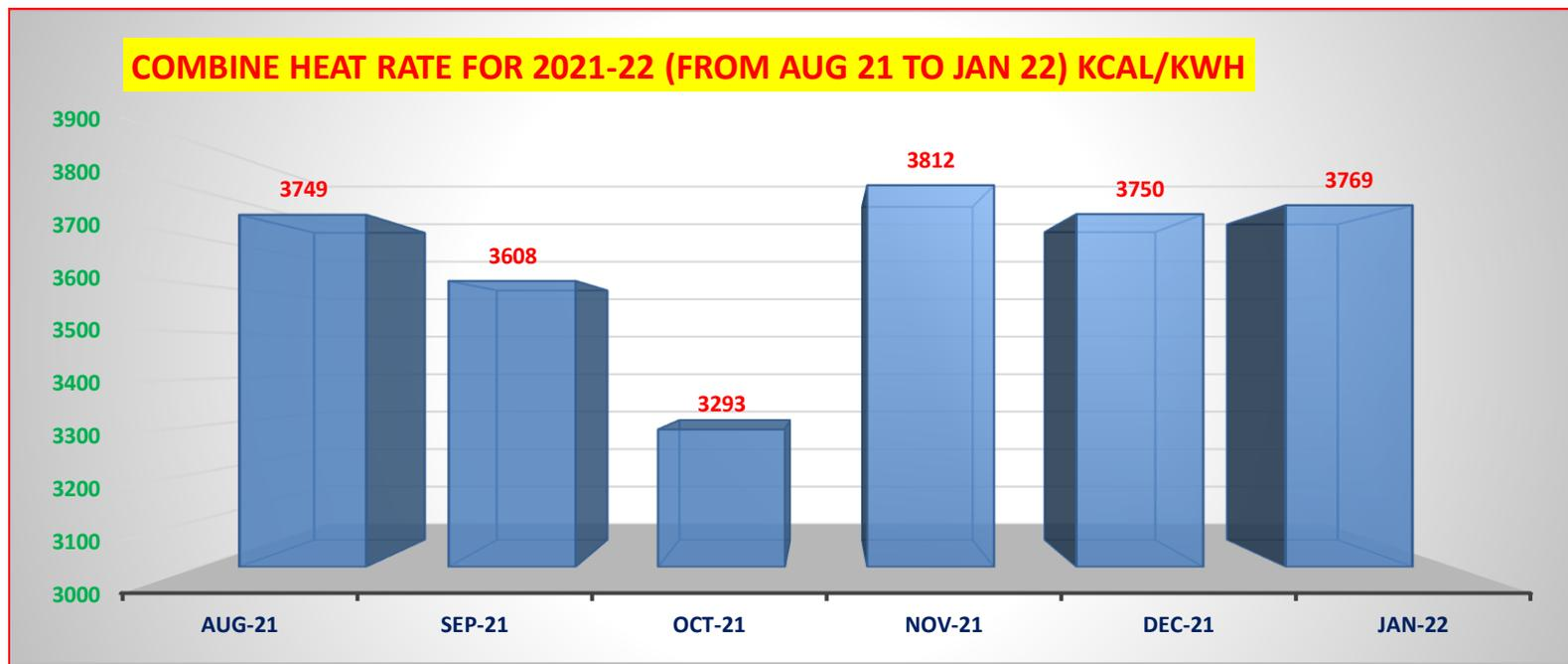
Observation : combine Heat rate of NTPS and NRPP for the year 2021-22 (FROM AUG 21 TO JAN 22) KCAL/KWH is depicted in above bar chart. Combine Heat rate is observed maximum in the month of November 2022 i.e., 3812 kCal/kWh and minimum in the month of October 21 i.e 3293 kCal/kWh . the Average heat rate for the year 2021-22(Upto January 20220 is found to be 3663 kCal/kWh.
