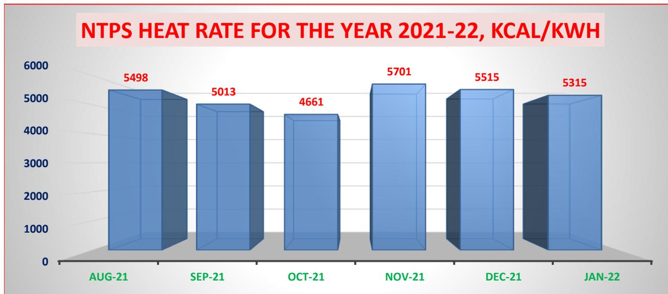
**Observation :** Heat rate for NTPS for the year 2021-22 (upto January 2022) is depicted in above chart. Heat rate is observed to be varying from 4661 kcal/kWh to 5701 Kcal/kWh. Heat rate is found to be highest in the month of November 2021 i.e., 5701 kcal/kWh and lowest in the month October 2021 i.e., 4661 kcal/kWh .
